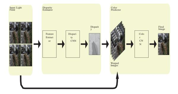
Figure 2 : Our system consists of disparity estimator and color predictor components which we model using two sequential CNNs. In our system, we first extract a set of features from the sparse input views. We then use the first CNN to estimate the disparity at the novel view. We then use this disparity to warp (backward) all the input views to the novel view. Our second CNN uses all the warped images along with a few other features to generate the final image
