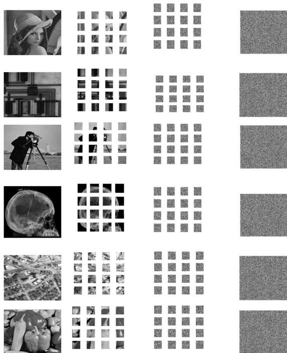
Encrypted Images of Lena, Circuit, cameraman, Human brain, Aerial and Peppers. First Column is Plain Images, Second is Block Dividation of images, Third is encrypted blocks of images and forth is fully encrypted images.
